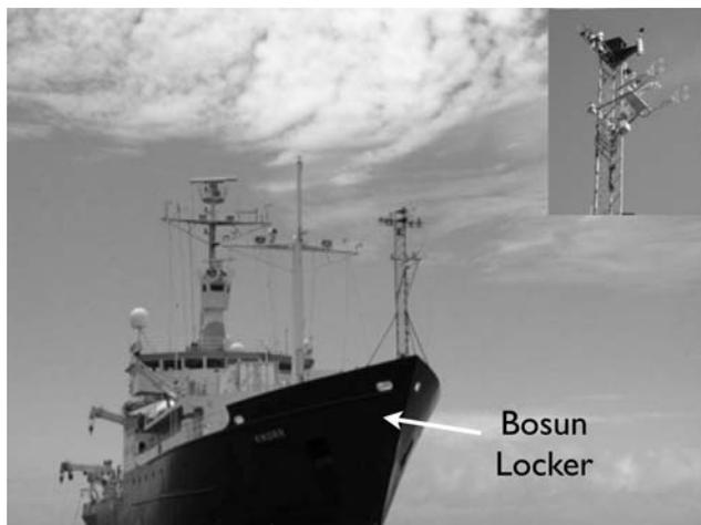
**Figure 1.** R/V *Knorr*. Anemometers, the motion sensor, GPS, and gas inlets were mounted to the bow mast (inset), approximately 14 m above the ocean surface. Gas analyzers were located in the bosun's locker, directly below the mast.
