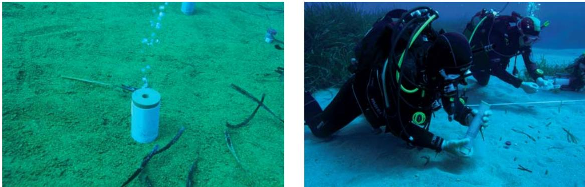
Fig. 5 – Taking sediment samples with push cores and Sarstedt tubes © HYDRA
