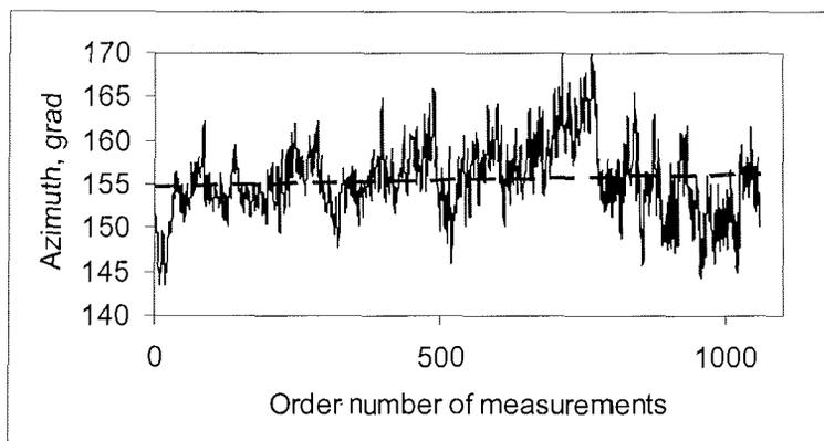
**Figure 5.3.2-1:** A diagram of measured azimuth fluctuations during the survey of the shoreface profile on the Bunge Land low part.
