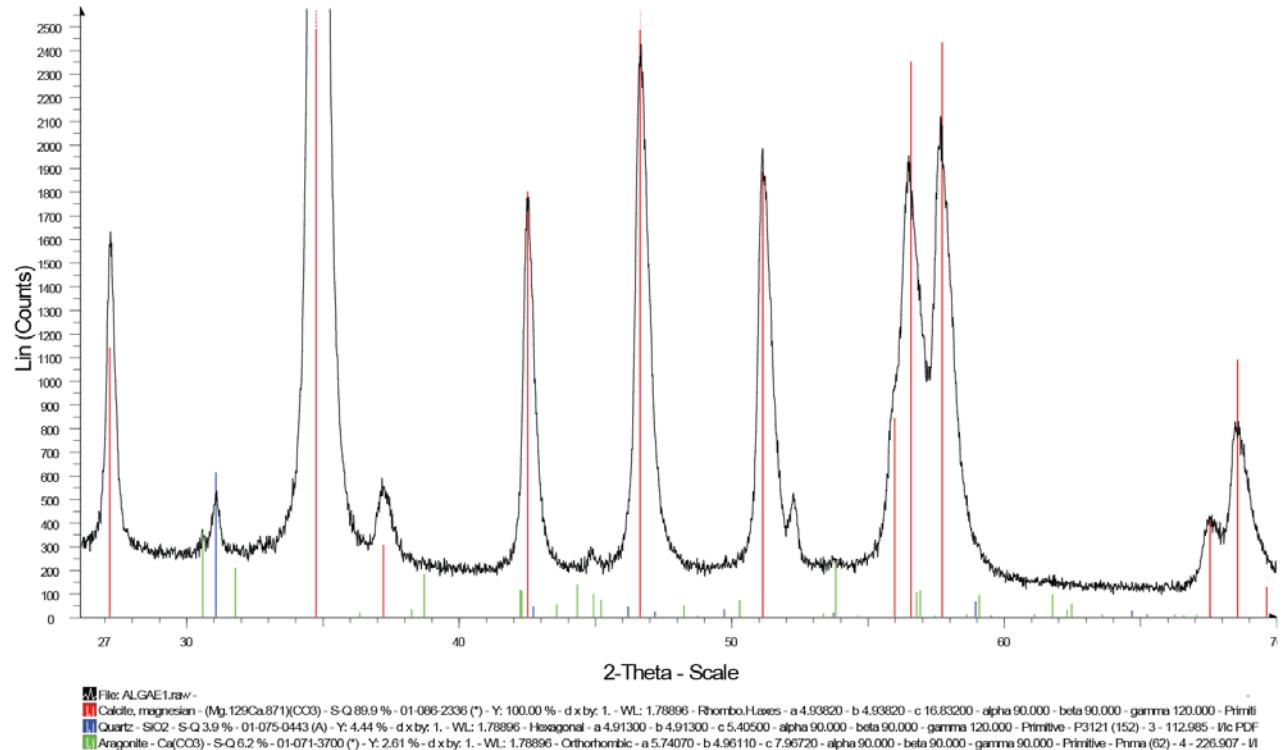
Fig S1: XRD spectrum, showing no sign of dolomite. This is important since in the tropical coralline algae *Porolithon onkodes* the presence of dolomite in the skeleton lowers the dissolution rates by 6-10 times (Nash *et al.*, 2012).
