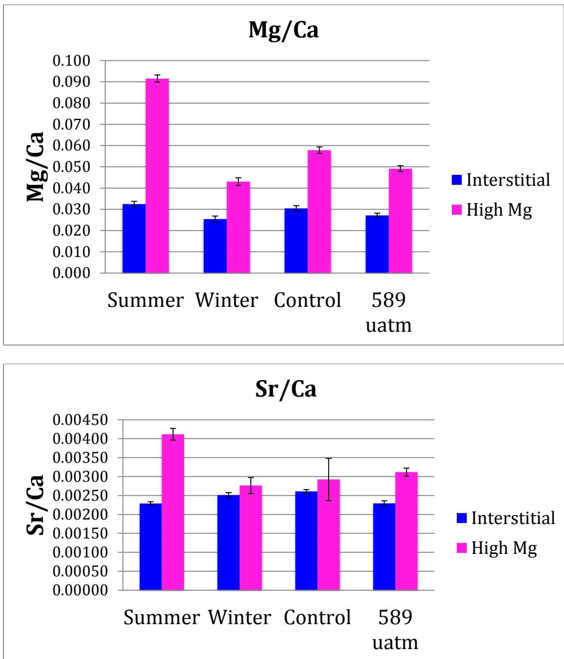
Fig S2: Mg/Ca and Sr/Ca ratios measured by NanoSIMS. The ratios were determined by extracting deadtime-corrected counts from regions-of-interest (ROI) in the ion images, and processing in a spreadsheet. Errors are expressed as the standard deviation
