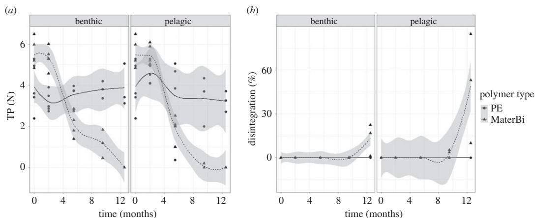
**Figure 2.** (a) Tensile properties (TP) and (b) disintegration of both polymer types in the benthic and pelagic habitat. Disintegration was measured as surface area loss in per cent. The curves and respective confidence interval (95%) were fitted using the method 'loess' in R. The number of replicates was reduced after 12.5 months owing to high fragmentation of the polymer.
