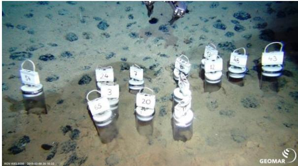
Sediment sampling with push corer.
