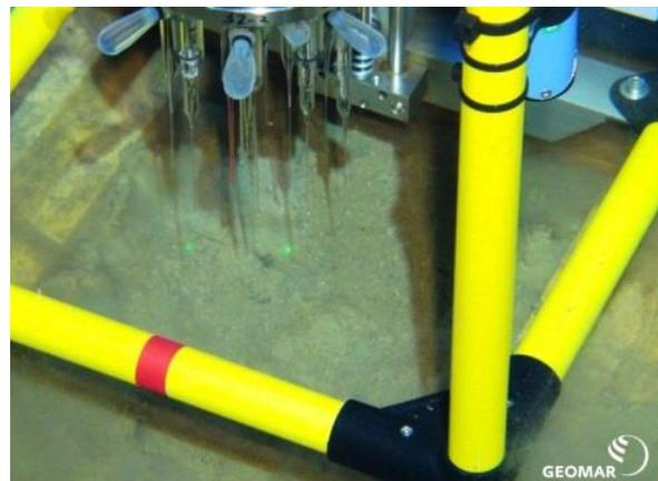
Microprofiler for the measurement of oxygen profiles with fine glass electrodes in the sediment.
