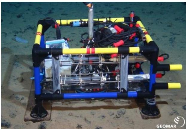
Benthic chamber for the determination of the oxygen consumption of the sediment.
