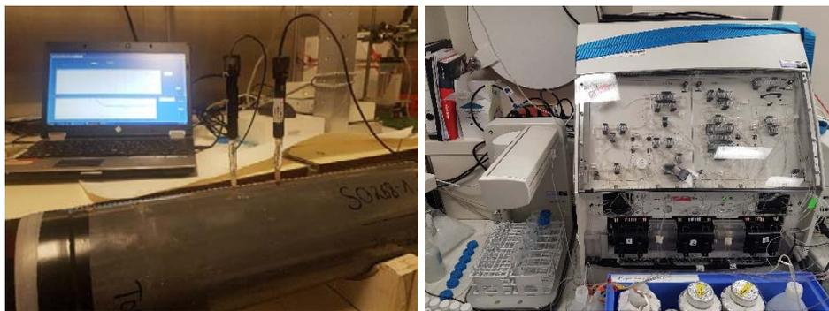
Photos (Jessica Volz): (left) Measurement of oxygen concentrations in long sediment cores using amperometric sensors. (right) Seal Analytical QuAAtro39 segmented flow analyzer used for the determination of nutrients in the pore water.
