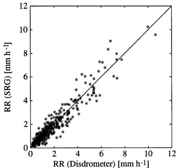
FIG. 5. Calibration of ship rain gauge (ordinate) against optical disdrometer (abscissa) from cruises with R/V *ALKOR*. Stars represent 8-min averages. Full line is the 1:1 relationship. The scatter is mainly due to sampling characteristics of the optical disdrometer and reduces with longer averaging times.
