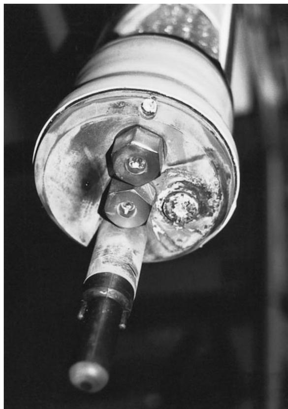
FIG. 2. End plate of dual release float No. 414 after recovery by FS *Poseidon*. The black hydrophone for the reception of acoustic signals with its extender pipe stuck through the released cylindrical ballast weight. The two hexagonal release blocks are displayed at the center of the photograph. On the right-hand side we see the strongly corroded valve screw. The instrument was under water for 15 months.
