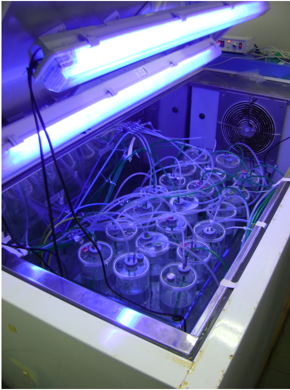
Figure 5: Experimental set-up for the CO 2 and temperature treatment: one of three freezer cabinets, which were assigned to each one target temperature level. The freezer held a water bath with 20 reactors, which were assigned to four pCO 2 levels. CO 2 gas was supplied via pipes from gas mixing pumps. Light from the top simulated Arctic summer light conditions for respective habitat depth of collected alga material ( 12 \mu\text{mol m}^{-2} \text{s}^{-1} for 24 h).
