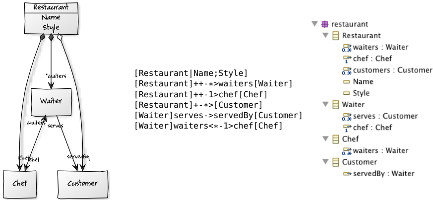
Figure 3.2. Different Representations of a Class Model: Diagram, Text and a Tree View (created with yUML ( http://yuml.me ) and Eclipse)
