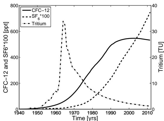
**Fig. 2.** Surface water input histories of CFC-12, SF<sub>6</sub> and tritium. For CFC-12 and SF<sub>6</sub> the atmospheric mixing ratios in ppt (Bullister, 2011) are assumed to be in 100 % equilibrium with the Mediterranean surface water. The tritium input history is based on observations and taken from R. Steinfeldt (unpublished data).
