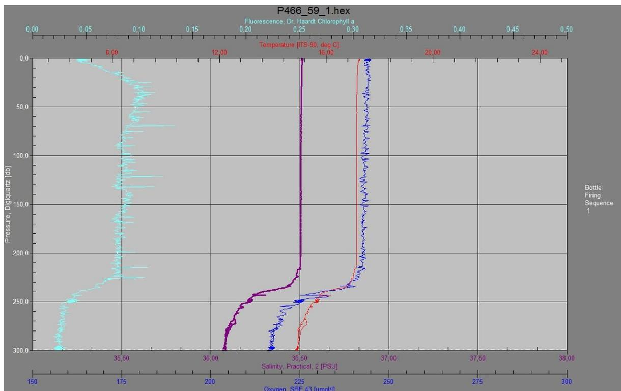
**Figure 3: CTD profile at station 59 showing homogenous mixed water layer down to about 250 m. (temperature = red, salinity = violet, oxygen = dark blue, fluorescence = light blue).**
