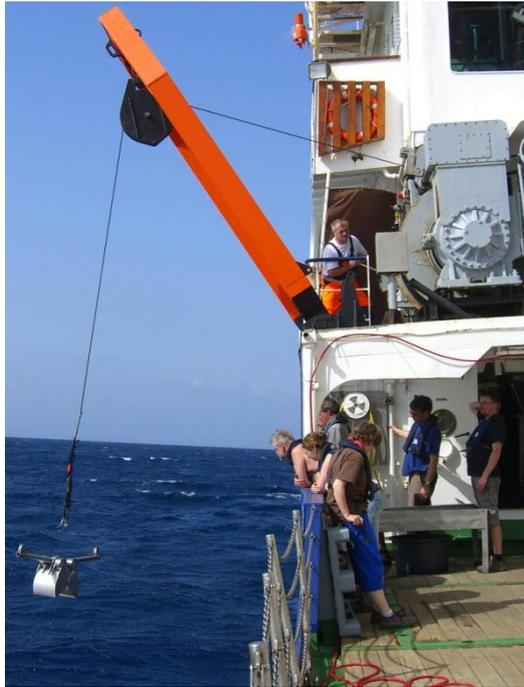
**Figure 2: Deployment of the van Veen grab during P466. Photo: C. Zinßmeister.**
