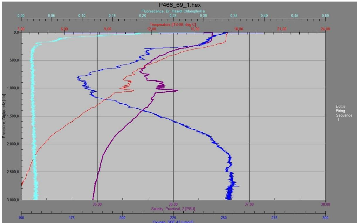
**Figure 4:** CTD profile at station 69 showing homogenous mixed water layer down to about 250 m, strong clines until about 600–800 m, the Mediterranean Outflow water at about 1,000 m and decreasing values of temperature, salinity until maximum measured depth (3,000m). (temperature = red, salinity = violet, oxygen = dark blue, fluorescence = light blue).
