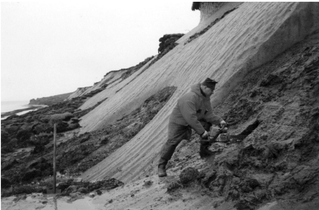
Figure 4.7-6. Coastal sediment and ice wedge sampling by chain saw (area of Mamontov Klyk, August 2003)
