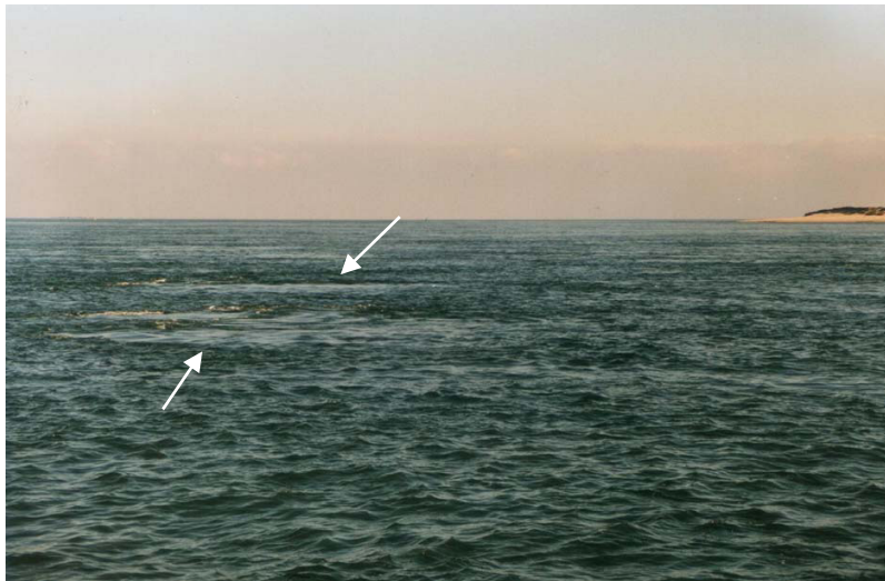
Figure 7. Handheld camera picture of turbulence patterns (marked by arrows) in the sea area of the Lister Tief acquired from on board the R/V Ludwig Prandtl at 1519 UT 15 August 2002 during flood tidal current phase.
