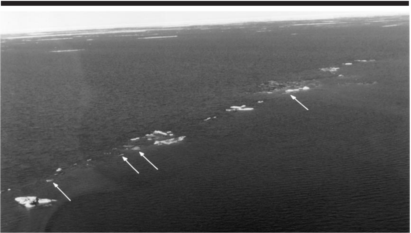
Figure 4. Aerial photograph of the shallowest segment of Dinkum Sands on July 15, 1979, viewing northwestward. Individual gravel mounds above sea level are dry, as marked by arrows. White objects represent a linear accumulation of brash ice grounded along the crest of the shoal.
