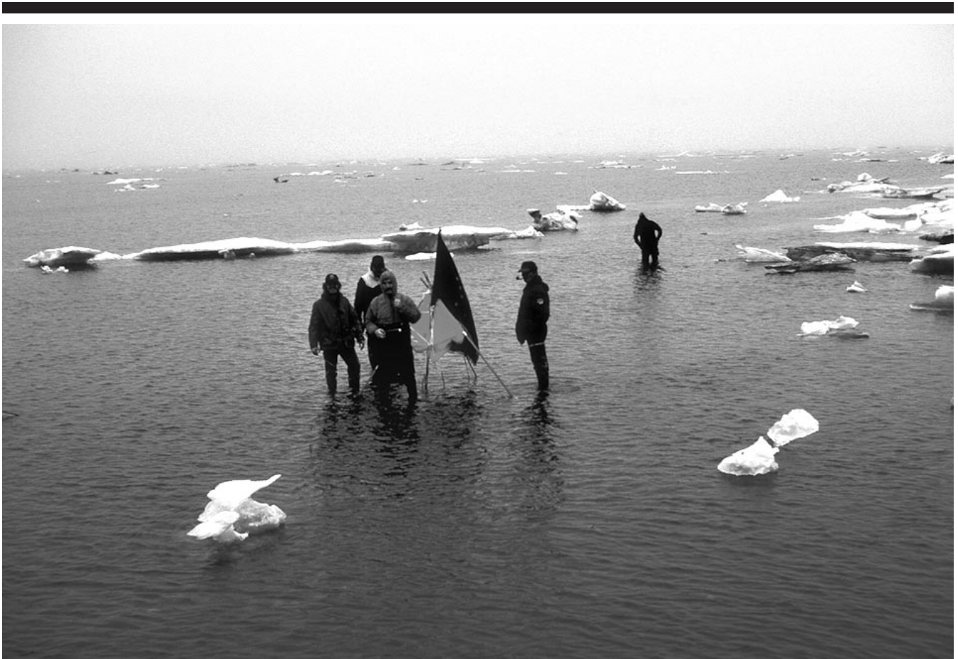
Figure 5. The highest point of Dinkum Sands surveyed during the previous winter as photographed from the grounded R/V Karluk with state and federal officials in waders on August 23, 1979. The minimum water depth at this time was about 20 cm. The flag marks a winter pile of sand and gravel with incorporated thin slabs of ice rising about 1 m above sea level 2 wk earlier, showing rapid changes in early summer.
