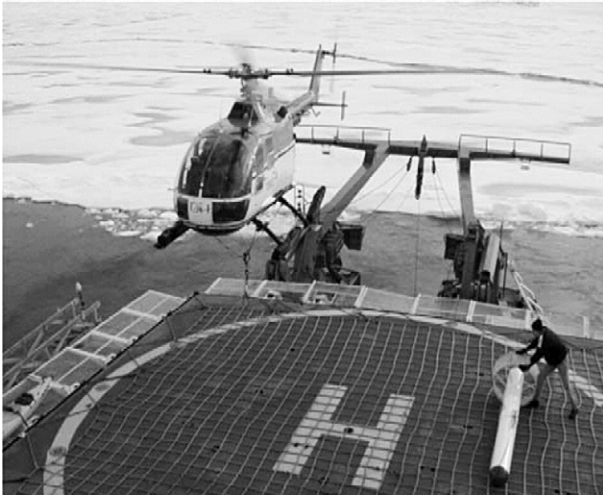
Fig. 2. AWI EM bird during take-off from the helicopter deck of an icebreaker, North Pole 2001.
