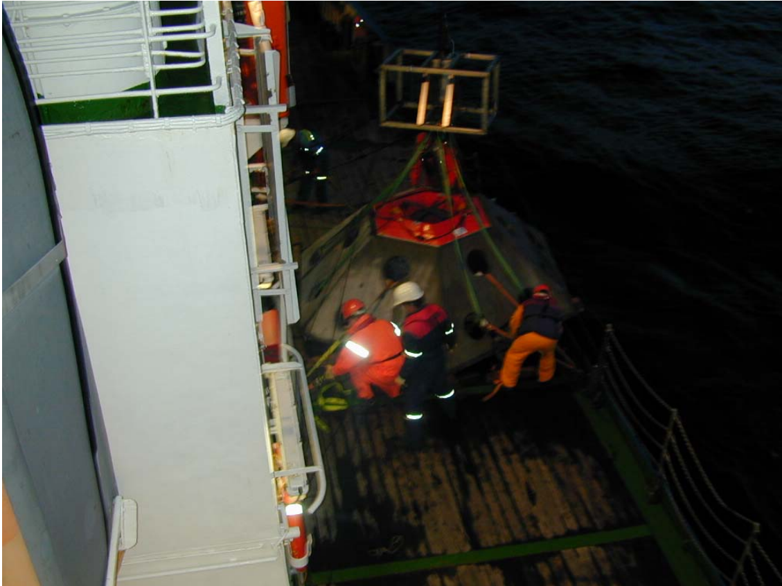
Fig. 5.1.2: shielded ADCP during the launching procedure during POSEIDON cruise P293; ADCP is housed below the orange top cap of the shield; double release inside the xxx shield; launching frame above the shield; the shield was viewed upside down on the bottom by the ROV's video camera system during P315.
