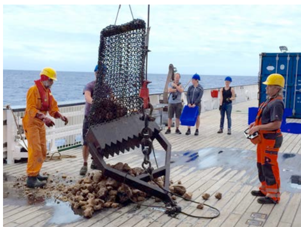
A nearly full dredge of pumice being emptied on deck. (Kaj Hoernle)
