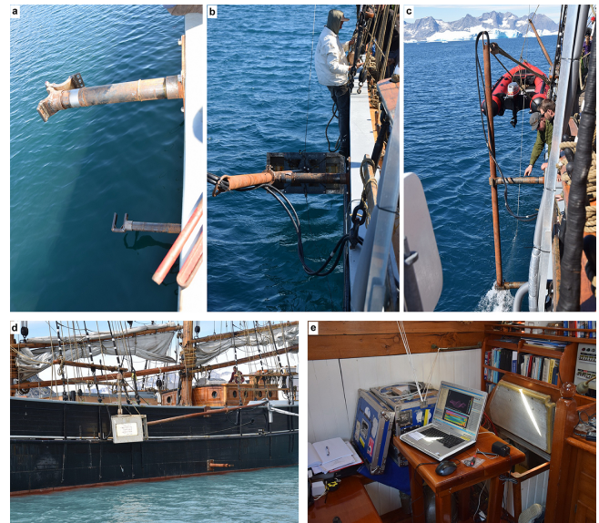
Figure 3. Deployment of the multibeam system onboard SS ACTIV using a clamp and a U-shaped clip (a–b). (c) The system during the surveying mode and (d) the system in the safe position used for transit. The multibeam system and computers were installed in the wheelhouse (e).
