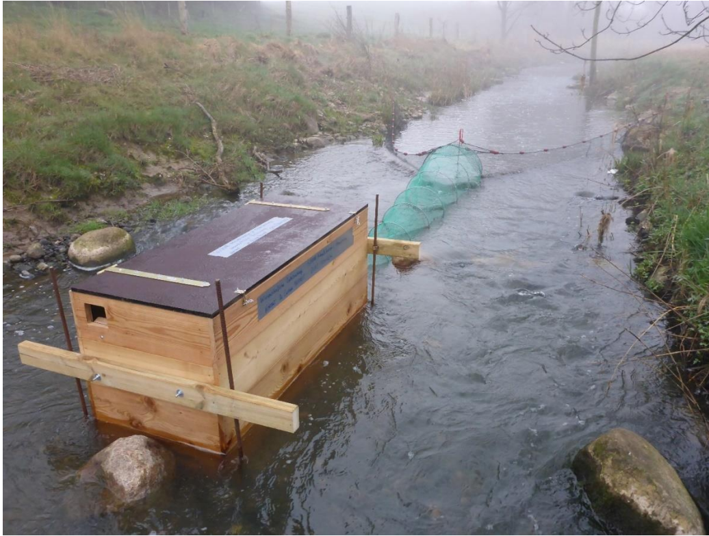
Figure 7: Smolt trap of the Lipping Au. The bow net covers the whole width of the stream concentrating the down moving fish in the centre where a creel net leads the fish to a self-made capture box
