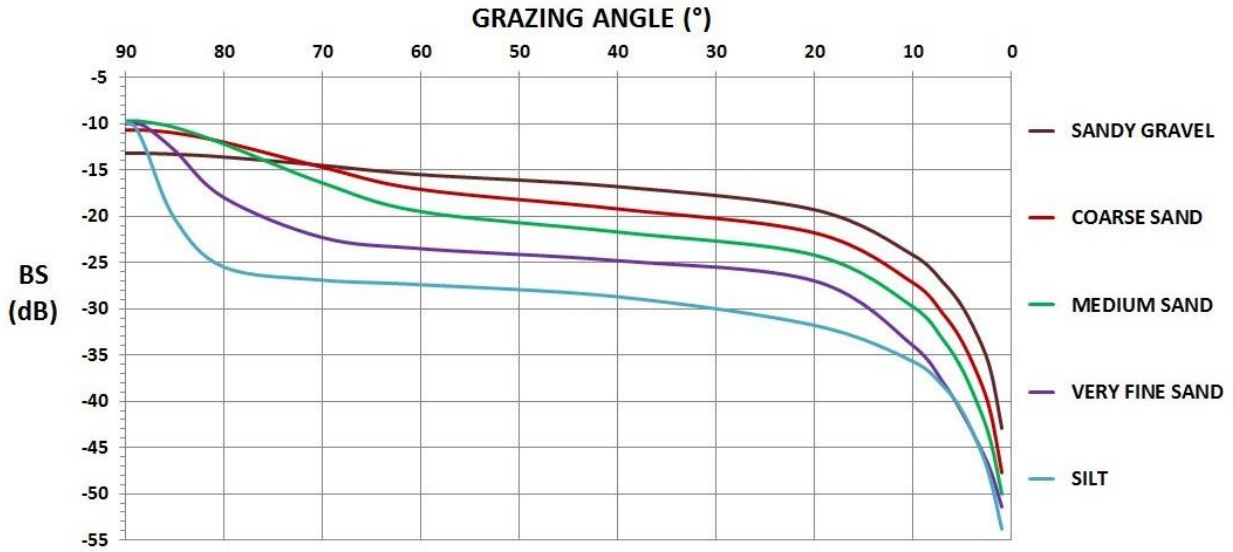
Figure 2.10: Prediction of angular response values of general sediment types using the APL model for 100 kHz frequency. (source: Lurton and Lamarche, 2015).
