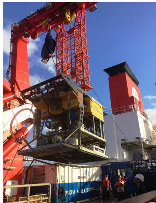
Right: LARS for deployment of ROV Kiel 6000 attached to the A-frame on the back deck.
