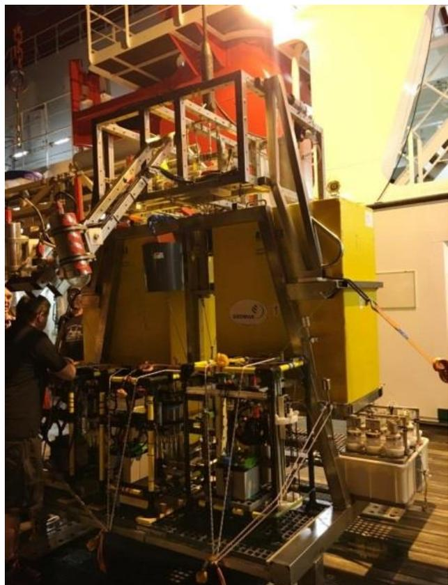
Right: Elevator-Lander with launcher on top.
