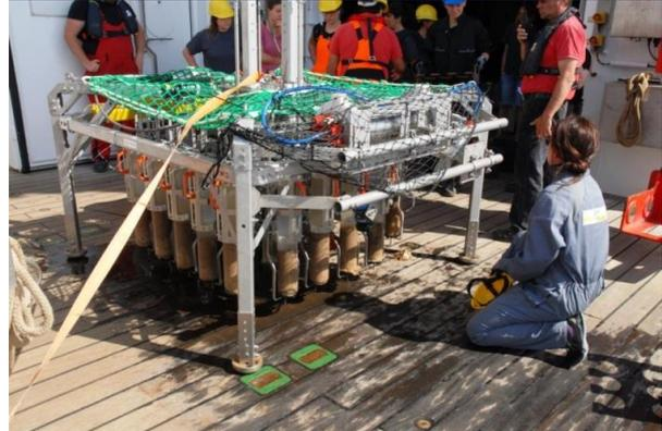
Preparation of the equipment (Elevator-Lander with Launcher, box corer and multicorer) on deck as well as the first video-guided deployment of the new multicorer.
