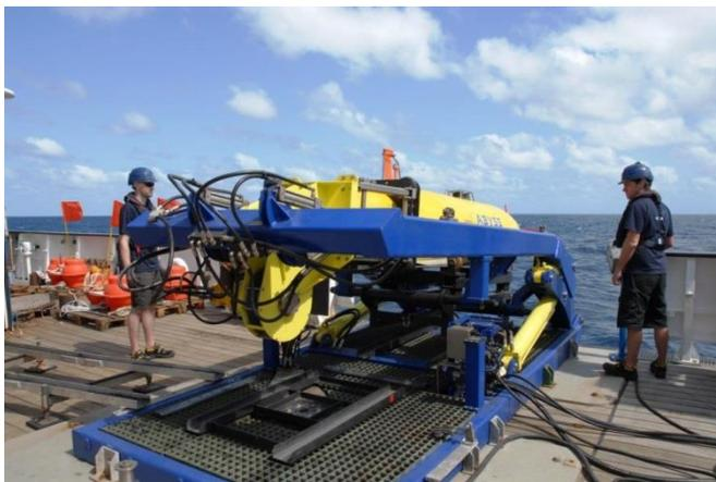
Launch and Recovery System (LARS) for deployment of the AUV ABYSS on the starboard side of RV SONNE.
