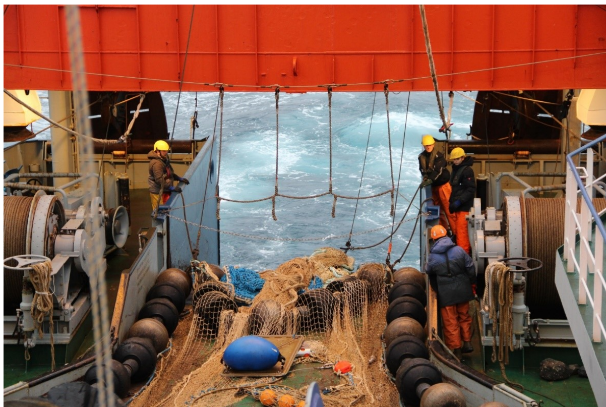
Picture 2.2: Deploying the BT140 (bottom trawl) net in Greenland autumn 2017
