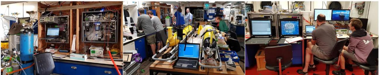
*Lab scenes: Automatic system for measuring CO<sub>2</sub> in surface water (left); gliders are being prepared for deployment in the geolab (center); the CTD watch is preparing for the next use of the CTD rosette system (right).*
