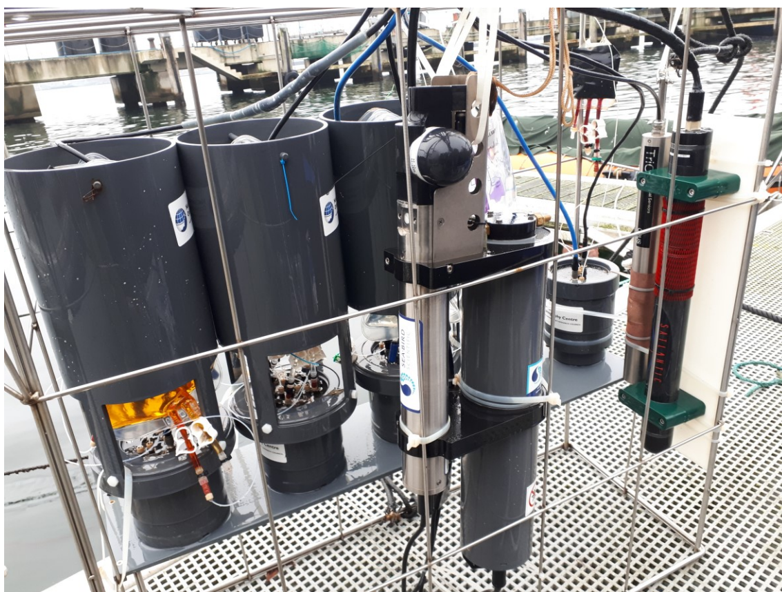
Figure 2.12: Deployment frame with LoC analyzers, optical nitrate sensors and SeapHOx attached (photo credit: M. Nehir).
