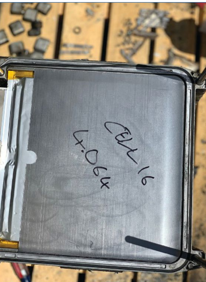
ESS cells 12 and 16 after exposure at 950° C.
