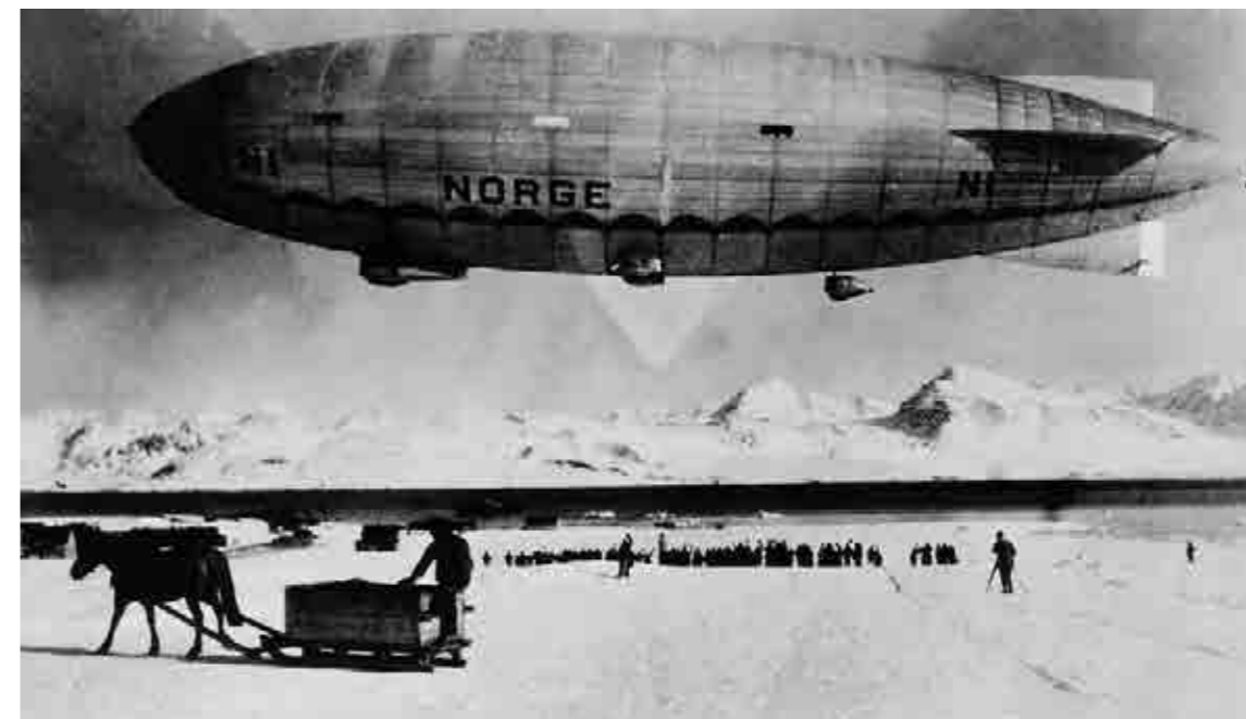
1.30 > The airship Norge , in which Roald Amundsen and his team flew from Spitsbergen over the North Pole in May 1926. It was 109 metres long and achieved a top speed of 85 kilometres per hour.
