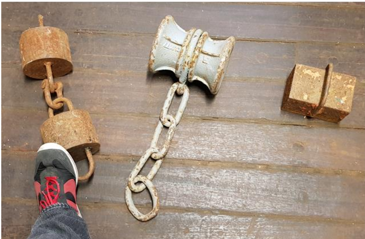
Figure 5.28: Typical elements of ship's rigging and hoisting devices can be used as a depressor weight of opportunity for deploying small robots, here ranging from 7 to 15kg, Finally, the middle block was chosen for the role.
