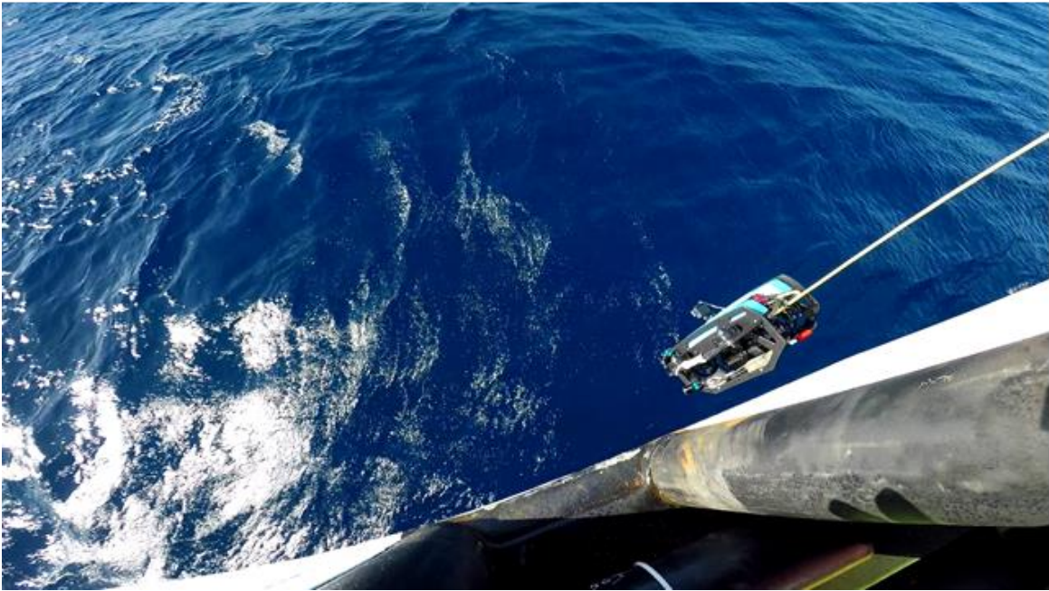
Figure 5.30: Deployment of the robot off the ship's bow included working with a significantly higher freeboard
