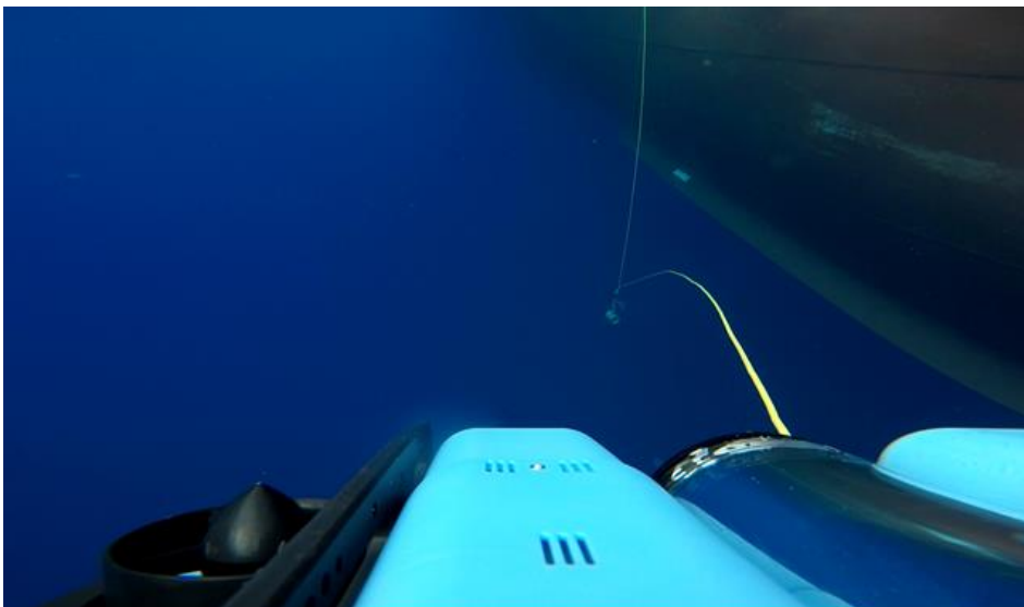
Figure 5.32: Images from the vehicle mounted camera show the position of the depressor weight and the free umbilical during deployment. Here, the depressor weight is lowered pass the bilge keels. In such videos it was also observed how the umbilical, rather taut due to the current, interacts with the vehicle
