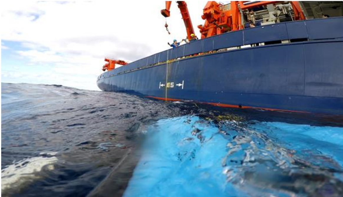
Figure 5.26: An important consideration during the initial stages of deployment of the robot is avoiding direct proximity of the ship while on the surface. This photo shows the arrangement of the crane used as an attachment point for the snap tackle and the depressor weight
