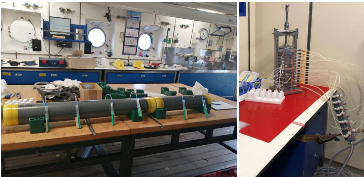
Figure 5.21: Rhizon sampling being performed in the Geolab of RV Meteor, and Geomar pore water press.
