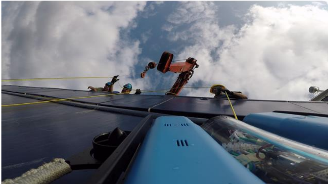
Figure 5.29: Deployment using a depressor weight slightly increases the complexity of the operation with the deck personnel required to control the winch or crane
