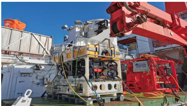
Figure 5.35: ROV and winch on the working deck (left); Nass-Labor serving as ROV control room (right)
