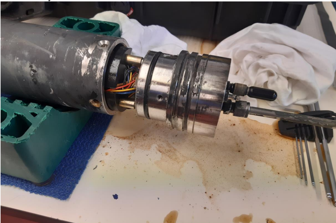
Figure 5.42: Observatory “ Christian ” recovered from the Carboneras fault in the Alboran sea. The housing has leaked over the years, seriously damaging the electronics.
