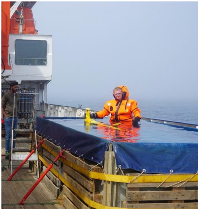
Test of an underwater glider vehicle in the test pool on deck of RV METEOR (Photo: J. Karstensen)
