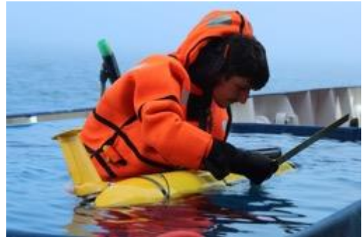
Félix Margirier (GeorgiaTech, USA) installing a wing on the underwater glider in a pool on deck RV METEOR. Photo: L. Blum
