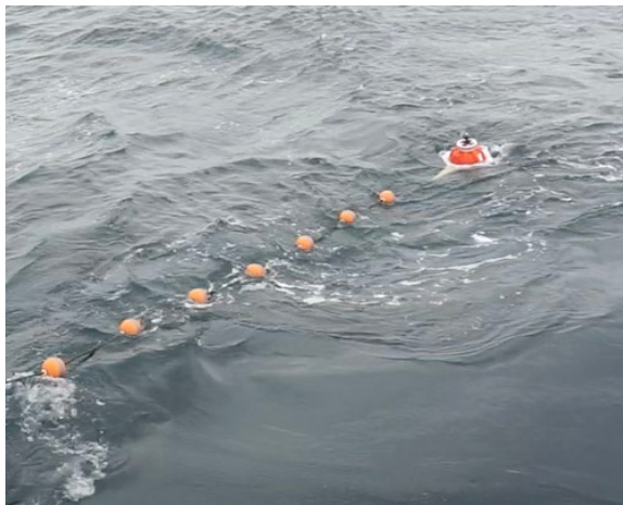
GEOMAR design Surface Telemetry module during the deployment of the K1 mooring. Photo: J. Karstensen
