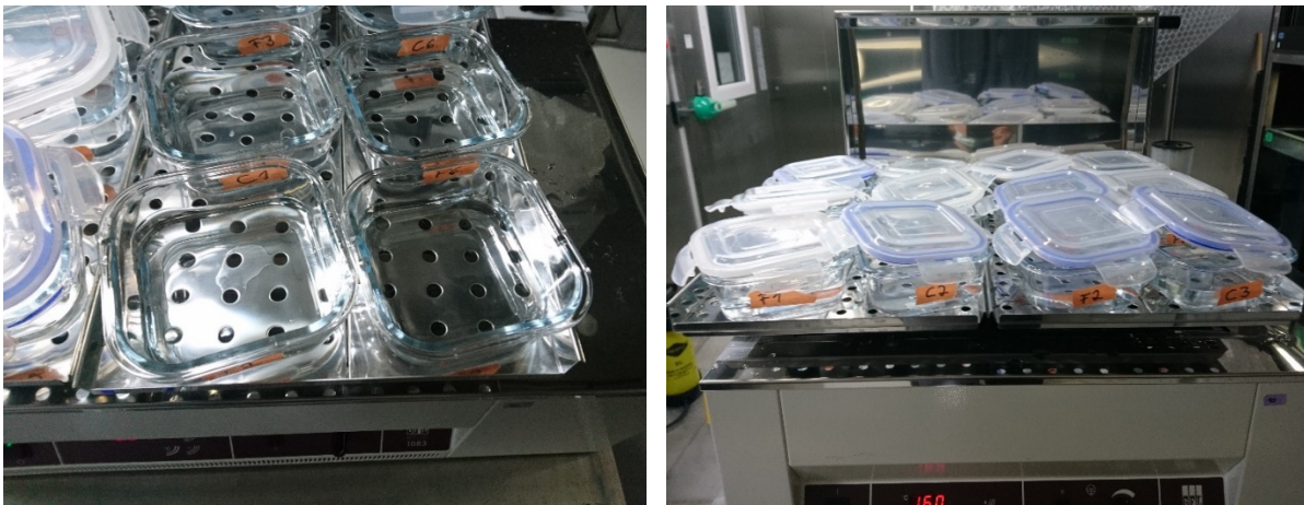
Figure S3. Experimental setup with square-shaped glass bowls placed in an angle towards the movement direction on the shaker to facilitate irregular movement of the water column (left). Bowls were kept loosely covered with lids, which were previously washed with filtered water and ethanol to prevent air-borne contamination during the experiment (right).
