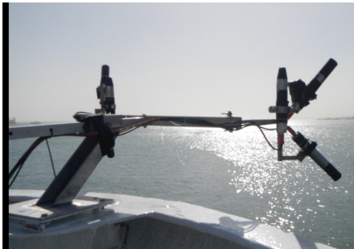
Fig. 3: Radiometers measuring optical properties of the ocean at the front of the RV METEOR. Photo: Shungu Garaba.
