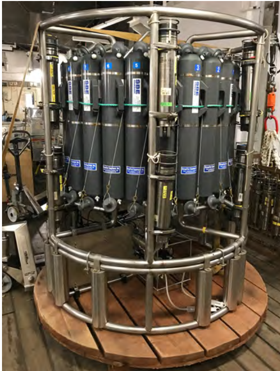
Figure 2: Releser mounted on the CTD rosette for a releser test. Foto: D. Lange, GEOMAR.
