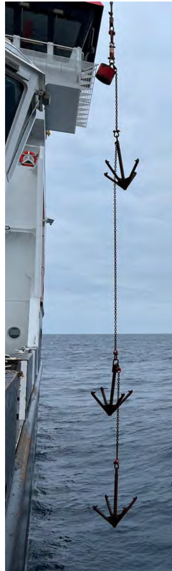
Figure 4: Anchors at the end of the chain and cable used for dredging. Photo: B. Bauer
