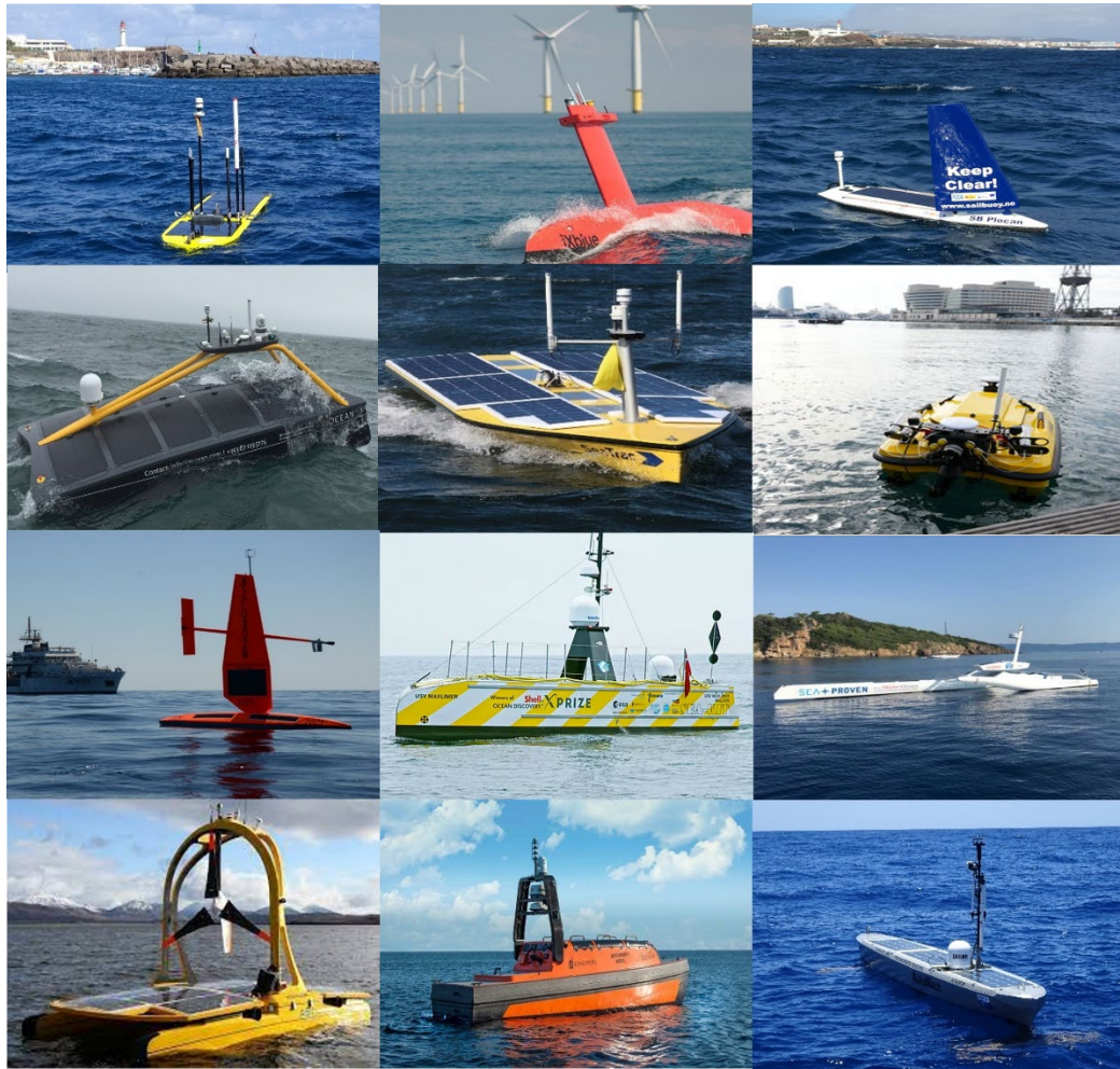
Figure 3. Some examples of the ASV technologies currently available for science and industry services. From left to right and top to bottom, WaveGlider (Liquid Robotics), Drix (EXAIL), Sailbuoy (Offshore Sensing), XO-450 (XOCEAN), (SeaTrack), (GPA-SeaBots), Explorer (Saildrone), SeaKit (Fugro), Spyrna (Seaproven), C-Enduro (L3 ASV), Sounder (Kongsberg Maritime) and AutoNaut-ASV (AutoNaut).
