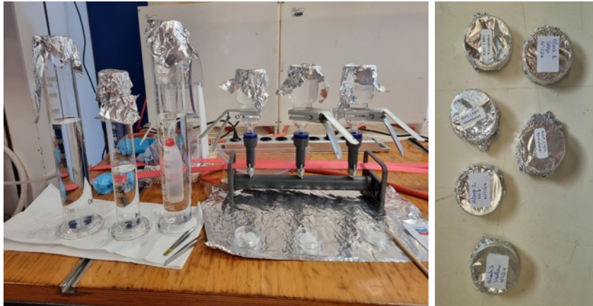
Figure 6. Glass measuring cylinders and aluminium packaging for the collection and storage of samples for microplastics. Photos: Leda Cai (CMMI).
