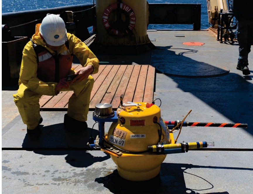
Figure 6. Image showing a JAMSTEC OBS being inspected upon recovery onboard Tully. Photograph by M.M. Côté. NRCan photo 2023-283.
