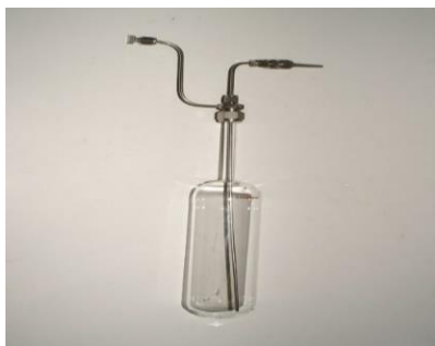
Fig. 5.15 Set-up of the sampling ampoules for CFC samples from the Niskin bottles.
