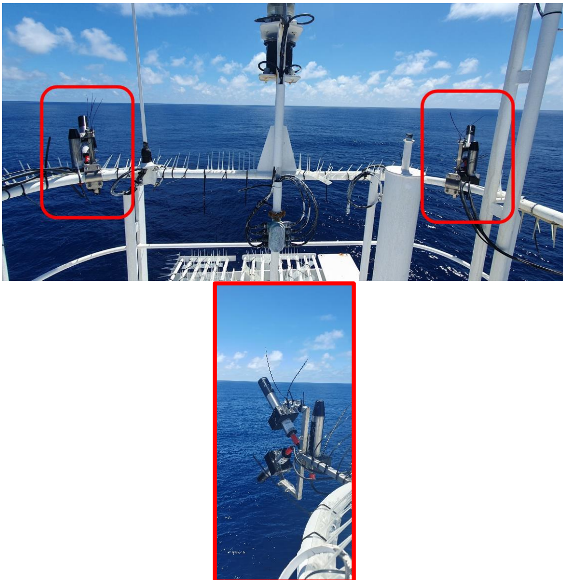
Fig. 5.3 TriOS hyperspectral radiometers and irradiance meters on top of the mast at the bow of RV SONNE during the cruise SO298.
