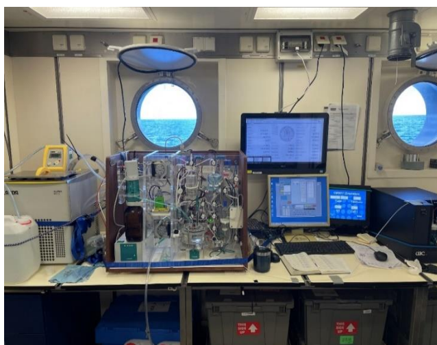
Fig. 5.14 VINDTA 3C lab set up for the determination of TA and DIC in the Climate Lab I on RV SONNE. From left to right: LAUDA water bath to provide a constant temperature of the samples previously and during measurement, container with NaCl rinsing solution, the VINDTA 3C for TA and DIC titration, PC, and the UIC.Inc coulometer for DIC determination. Below the table: grey boxes with CRMs.
