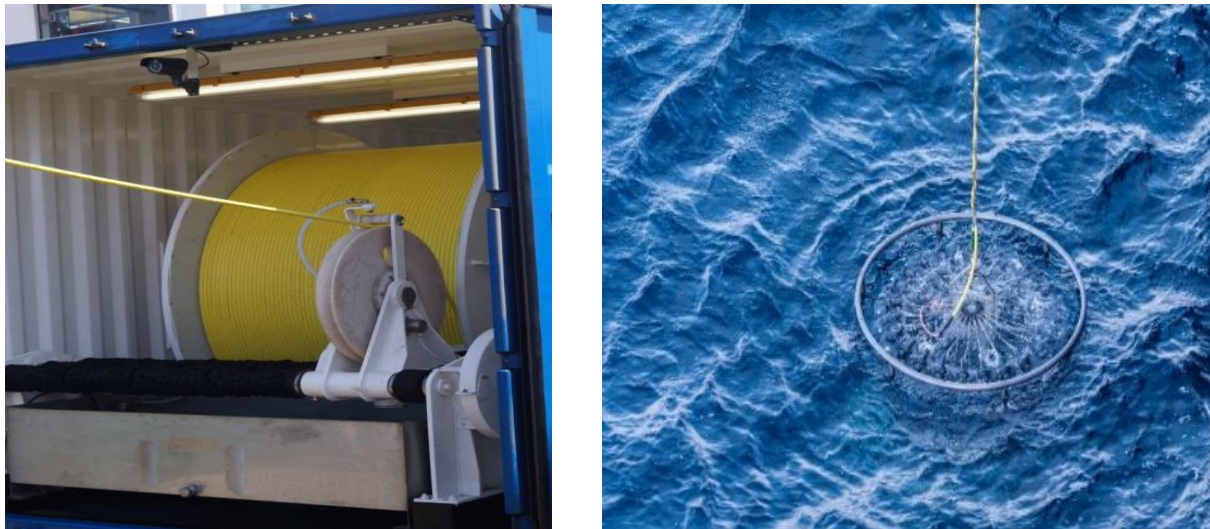
Fig. 5.1a Left: Winch with Kevlar conducting wire. Right: Deployment of titanium CTD frame. Photo E. Achterberg (left) and C. Rohleder (right).
