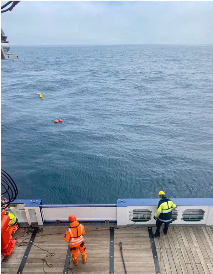
After being released from its anchor, the mooring shoals until it reaches the surface. Once spotted on the surface, recovery can start (Photo: Fehmi Dilmahamod)
