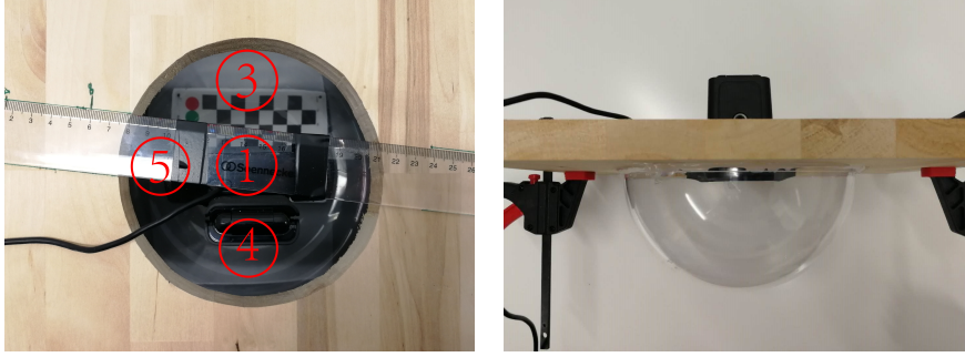
Figure 2.11: Experimental settings of the webcam with an acrylic dome. Left: Top view with test positions, Right: Side view.
