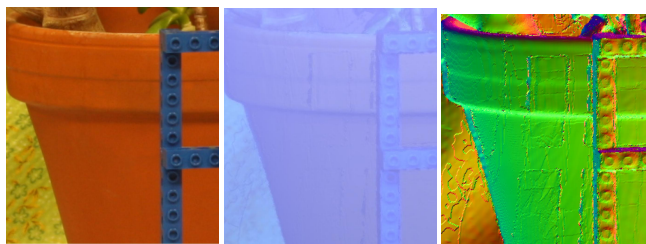
Figure 3.21: The slight noise present in the depth map becomes more noticeable when subjected to spotlight shading. From left to right: In-air color image, Deep sea synthesis, and Normal map.
