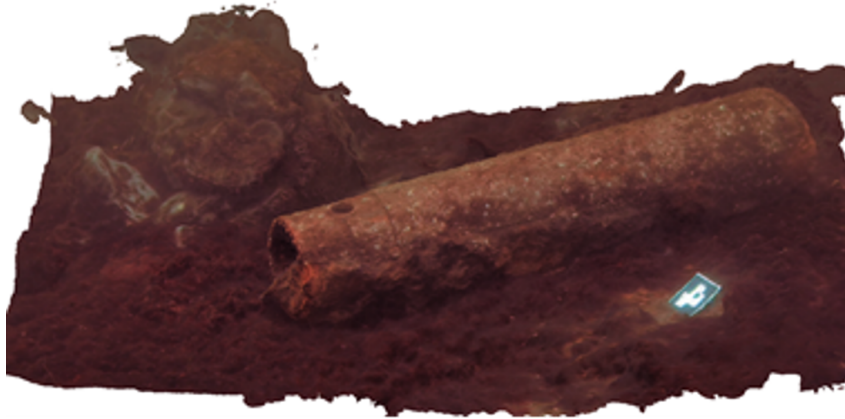
Figure 5.4: Reconstructed 3D model of a torpedo in the Baltic Sea via proposed approach.
