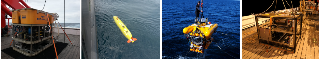
Figure 1.2: Examples of four different types of platforms used for deep-sea mapping. From left to right: ROV (GEOMAR KIEL 6000), AUV (GEOMAR ABYSS Tiffany), HOV (GEOMAR JAGO) and towed platform (OFOS frame).
