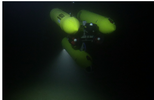
Figure 1.1: GEOMAR AUV ANTON (Girona 500) performing subsea visual mapping tasks in the darkness with its own lighting offshore. The co-moving light source creates a light cone in water, illuminates the seafloor non-homogeneously and forms up an artificial pattern in the image.
