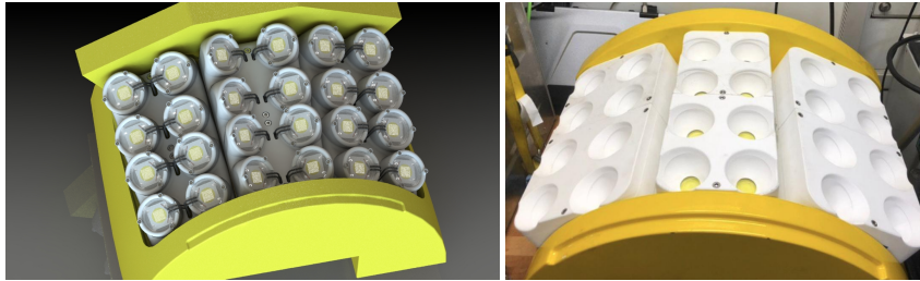
Figure 5.11: Left: Technical drawing of optimized LED configurations for 4m flying attitude mission in the Central Pacific. Right: Corresponding 3D printed LED rig bases. Courtesy: Emanuel Wenzlaff.
