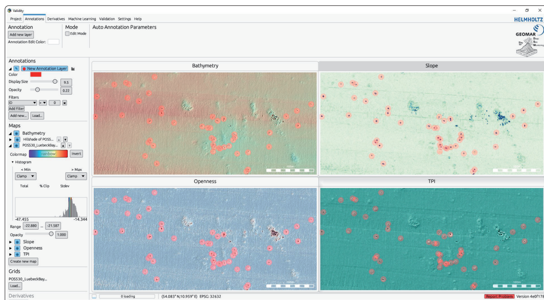
Fig. 3: Screenshot of the ValidTy software showing munition piles and single objects in Pelzerhaken. The integrated study of several map views in parallel and the very fast computation of derivatives and interactive changes (e.g. radii of the TPI or openness calculation) as well as the auto-aim option for annotation of single targets support easier and faster annotation
