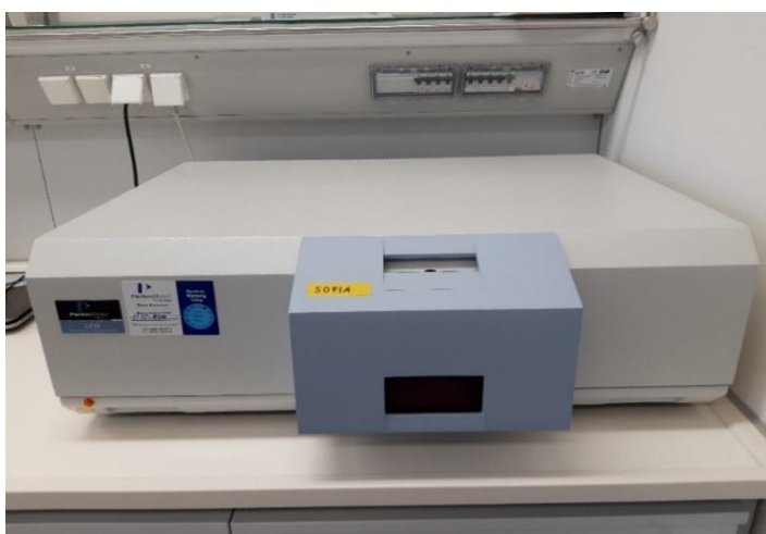
Fig. 5.4.2 Hyperspectral Fluorometer and resulting Excitation-Emission-Matrix (EEM)
