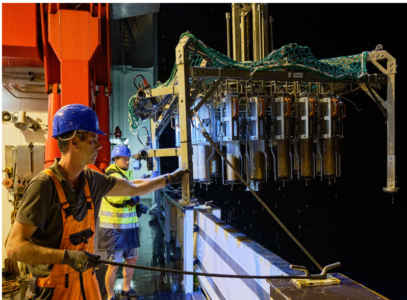
Fig. 5.6.1 Recovering the 20-liner Multiple corer equipped with video camera.
