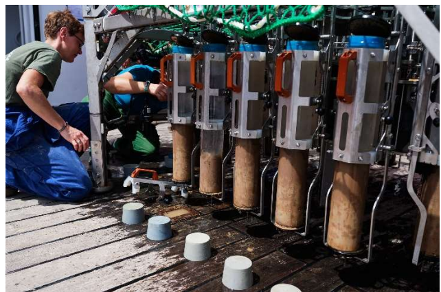
Fig. 5.14.1 Left: Deployment of the multicorer from RV SONNE (picture: Mirja Bardenhagen). Right: filled sediment cores arrived on deck (picture: Time Kalvelage).
