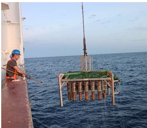
Fig. 5.14.1 Left: Deployment of the multicorer from RV SONNE (picture: Mirja Bardenhagen). Right: filled sediment cores arrived on deck (picture: Time Kalvelage).
