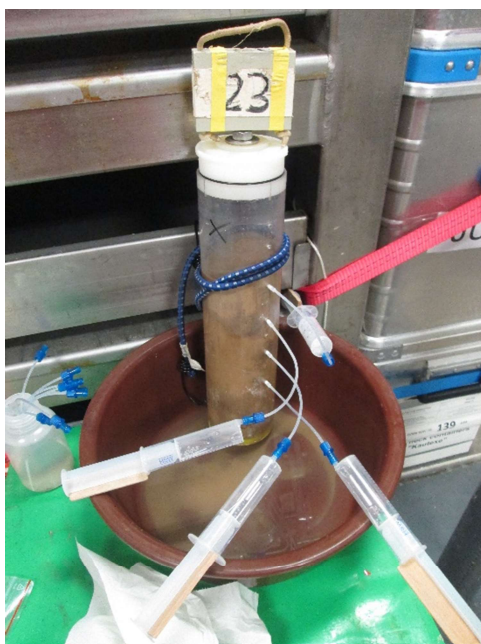
Fig. 5.14.8 Rhizon pore water sampling for Me-L analyses (picture: SO268, Sophie Paul).
