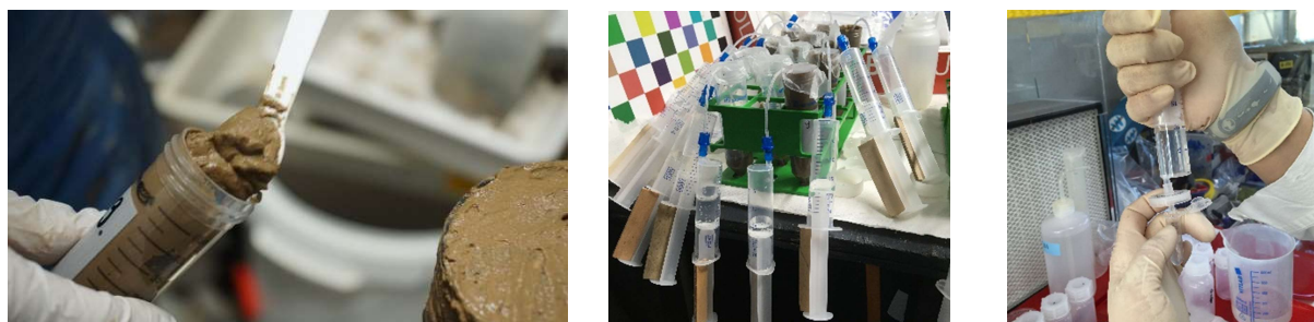
Fig. 5.14.7 Sediment sampling from core slices in the cold room (left), pore water extraction using rhizons (middle), syringe filtration of centrifuged pore water for alkalinity measurements (right). Pictures from cruise MANGAN2021: K. Schmidt (middle and left) and T. Aigner (left).
