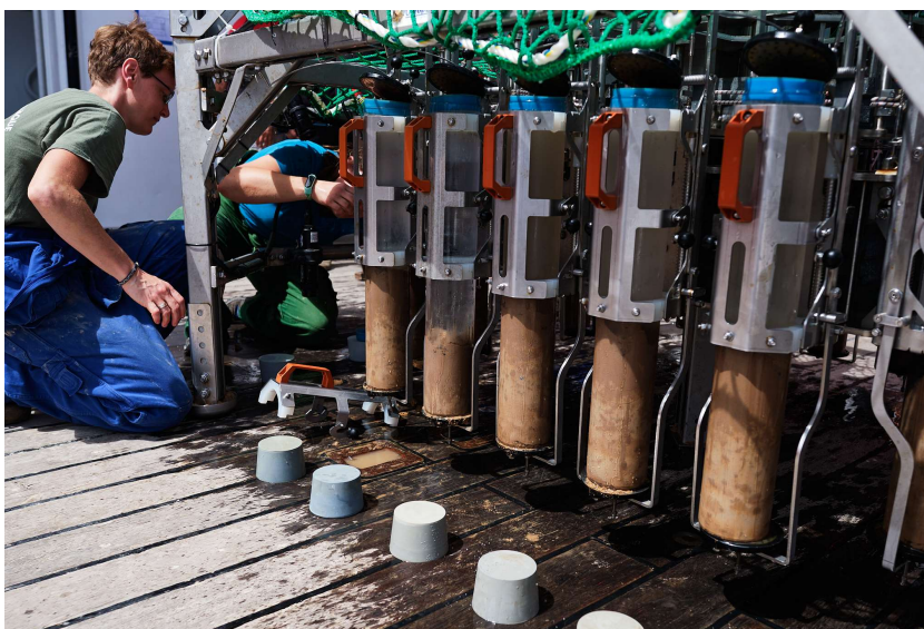
Fig. 5.6.2 Retrieving cores from the 20-liner Multiple corer on deck.
