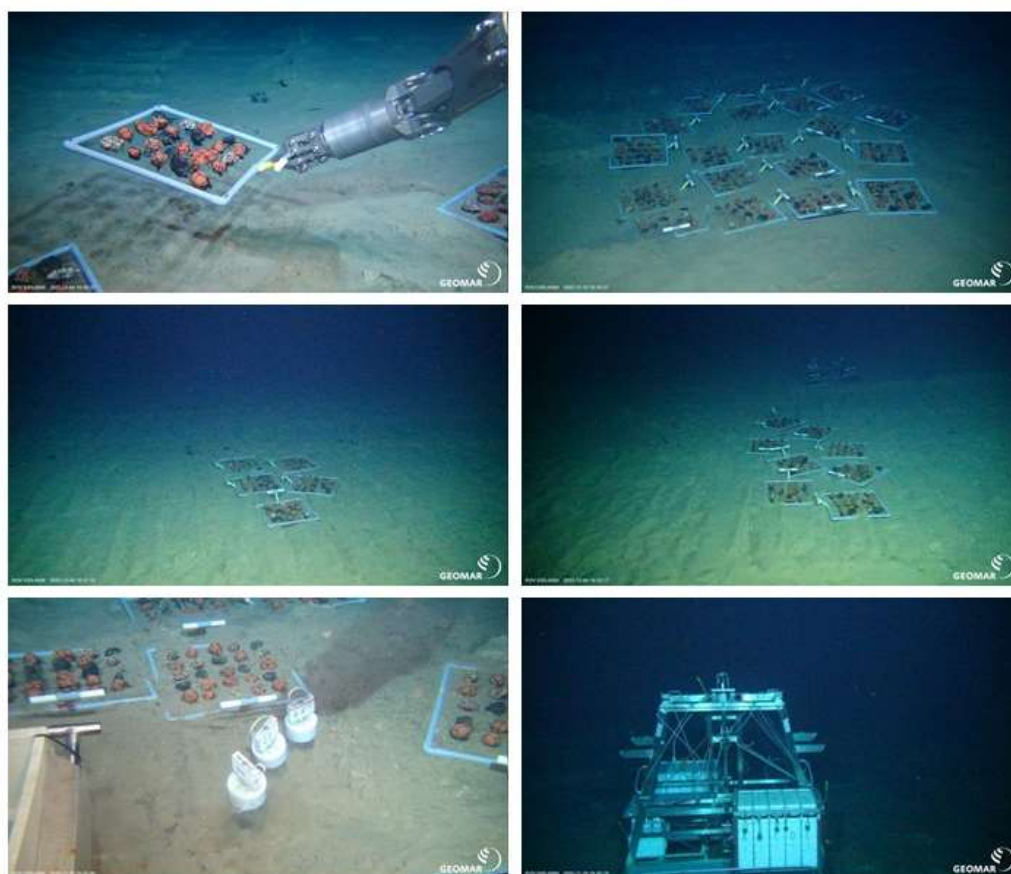
Fig. 5.17.8 (from left to right). Deployment of frame by ROV arm. New deployed frames in BGR area. New deployed frames in GSR area. New deployed frames in GSR area. Pushcores in frame inprint. Elevator with frame recovery boxes.
