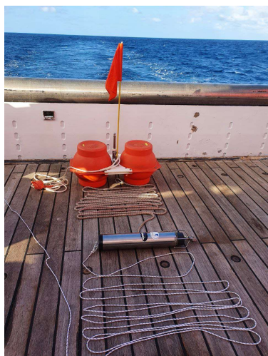
Fig. 5.2.2 (Left) Transponder setup on deck; (right) Photomosaic Abyss0371 provided on the GEO-Server.
