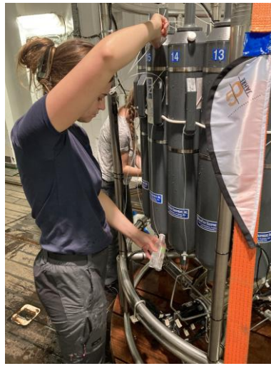
Fig.2b: Emptying the water samples from the different depths from the respective Niskin bottles.
