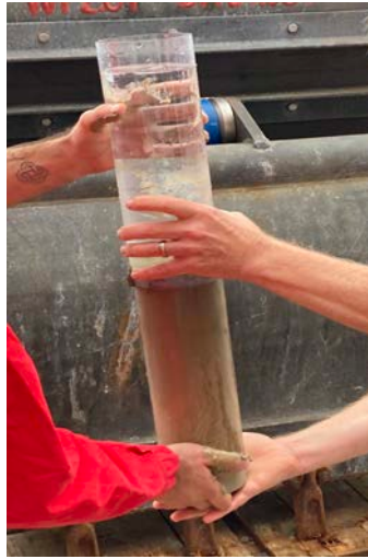
Abb.1b: The pipes with the excavated sediments are carefully recovered. The top 30 cm are still filled with the original ocean bottom water from a depth of several thousand meters. Photo: J.G.
