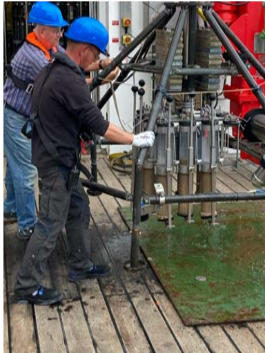
Fig.1a: A successful MUC filled with deep-sea sediment comes back on board. Science (left) and ship's crew (right) work hand in hand. Photo: J.G.
