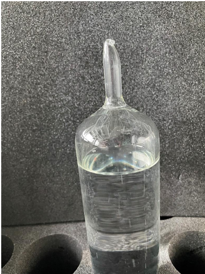
Figure 2.2: Picture of a flame sealed ampoule showing the headspace filled with pure nitrogen.
