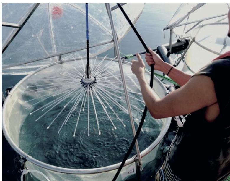
Figure S2. Spider used to facilitate the uniform enhancement of alkalinity during addition. By moving the device up and down the water column at a consistent speed during the injection process, alkalinity is evenly dispersed throughout the water. Photo source: Ulf Riebesell.
