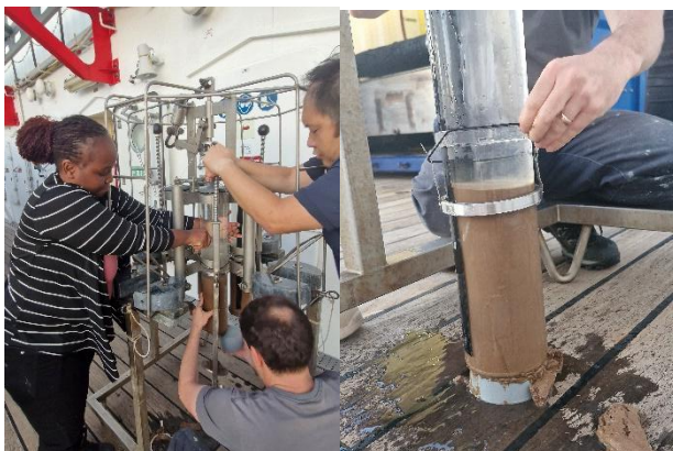
Fig. 5: Deep ocean sediment samples obtained at station 19. Team collecting sediments from the mini MUC, and close-up of core. Photo E. Achterberg.
