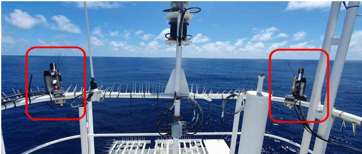
Figure 2: Radiometer on the mast at the front of the RV Sonne. Photo Brandy Robinson.
